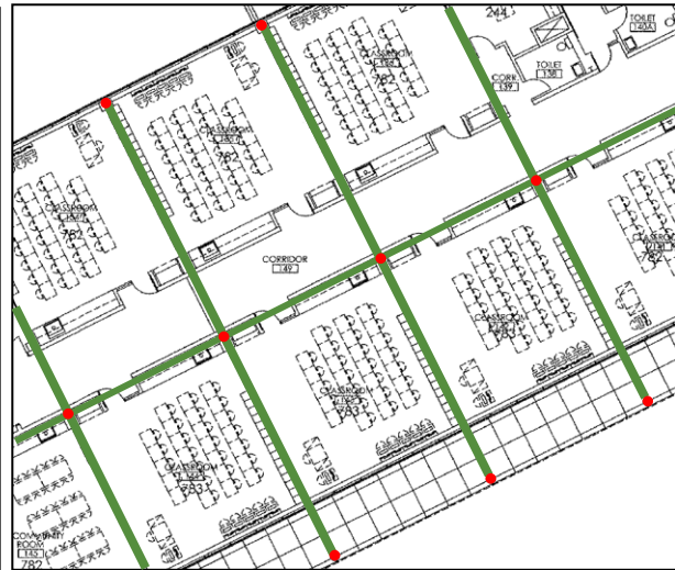
Figure 2: Modified Structural Grid
